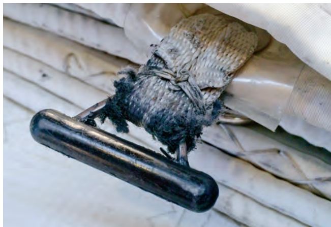
TOP: Chafe is one of the worst offenders for sail damage. Check for areas that may need re-stitching. ABOVE: The webbing on a main's slides takes heavy punishment and will need replacing from time to time.
