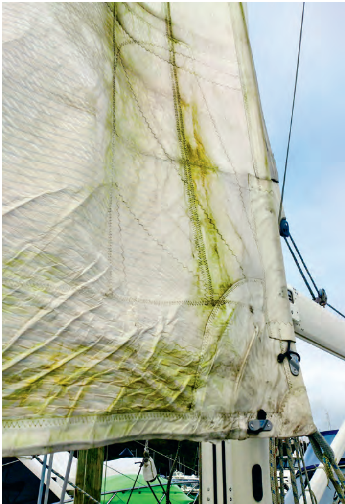
Serious algae damage - an entirely new sail might be required.
