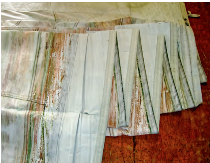
Lack of use makes a furling sail the ideal environment for mildew to prosper.
