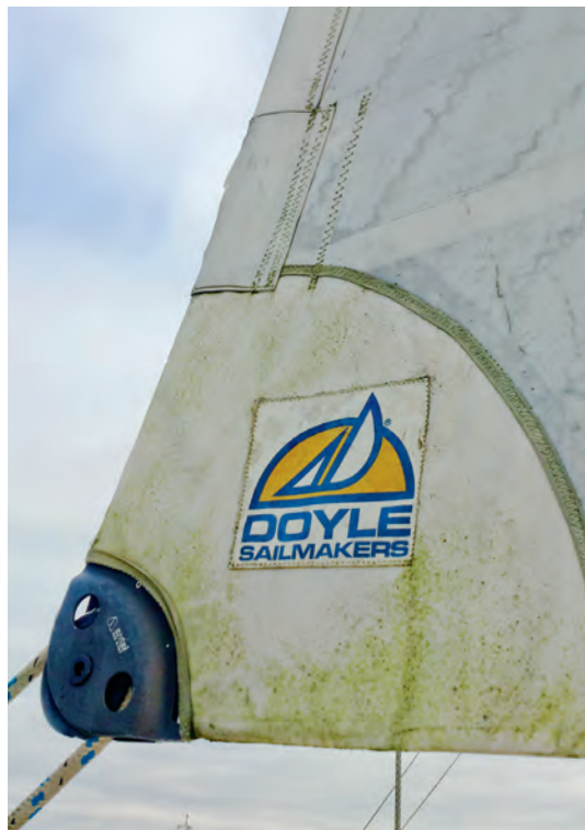
Another example of mildew and algae - and a seriously weakened clew.
